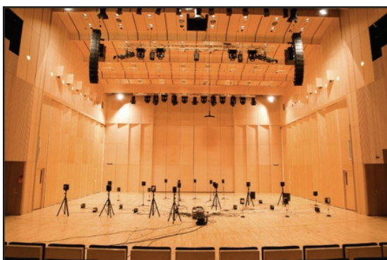
Figure 2: The recording of music emitted by the loudspeaker orchestra in a concert hall. The six microphone signals are converted to B-format, which is furthermore processed with DirAC for 16-channel loudspeaker reproduction [2].
