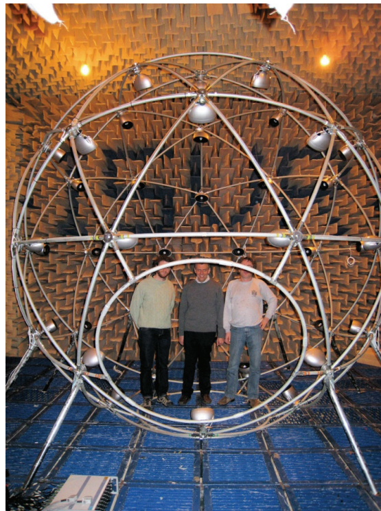
Figure 18: ISVR's spherical playback system
