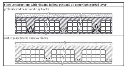
Figure 2 – Types of beam and clay block floors shown in ISO 12354-2:2017.
