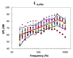
Figure 1 – Distribution of experimental data of impact sound pressure level measured for 40 bare floors in hollow-pots and concrete (in-situ).
