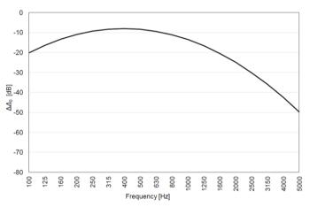
Figure 4 – Normalized correction spectrum  $\Delta\Delta_0$  to calculate contribution  $\Delta_0$  to be applied to  $\Delta L$  data measured on a concrete floor to estimate improved impact sound insulation on a CLT floor (values at 4000 Hz and 5000 Hz extrapolated from measured value up to 3150 Hz).
