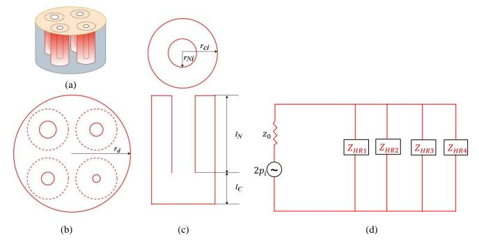
Figure 1 – (a) Physical model of the metasurface. (b) Top view of the metasurface and (c) schematic diagram of the HRIN, where  $l_N$  is the neck length,  $l_C$  is the cavity beyond neck length,  $r_N = d_N/2$  is the neck radius  $r_C$  is the cavity radius and  $r_d$  is the radius of the metasurface structure. (d) Equivalent electro-acoustic circuit of metasurface, where  $Z_{HRi}$  is the acoustic impedance of the *i*<sup>th</sup>HRIN.
