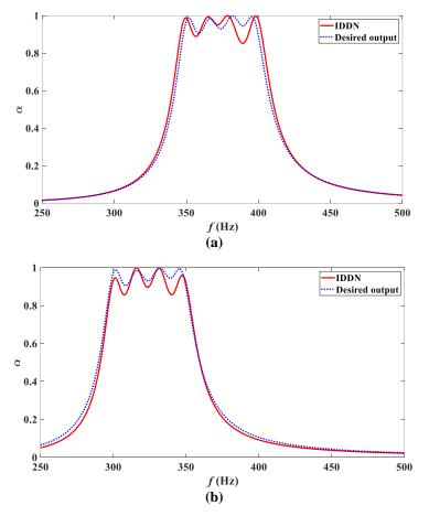
Figure 4 – Comparison between the desired absorption characteristics and the absorption characteristics generated using the geometric parameters predicted by IDDN method for metasurface models (a) S1 and (b) S2.
