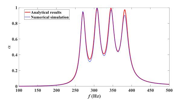
Figure 2 – Sound absorption characteristics of metasurface from analytical and numerical simulations. The dimensions of the metasurface are given in Table1.
