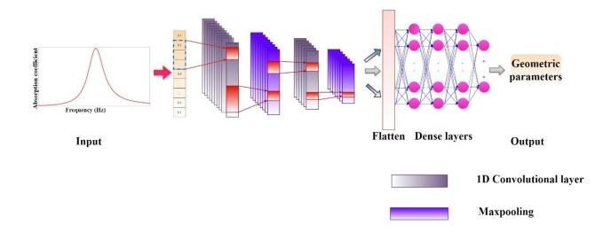
Figure 3 – Schematic representation of DNN architecture.
