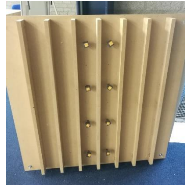
Figure 12 – Setup of the vibration absorbers installed on the joist structure.
