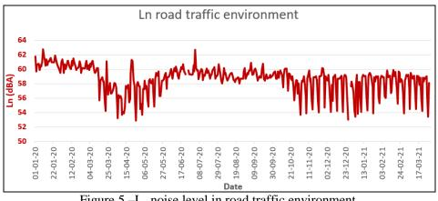
Figure 5 – L<sub>n</sub> noise level in road traffic environment.
