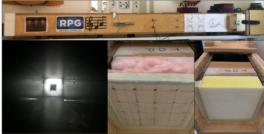
Figure 4 – 16 cm 2 impedance tube (top). Four-microphone measurement system (bottom-left). Test sample S5 (bottom-middle). Test sample S7 (bottom-right).
