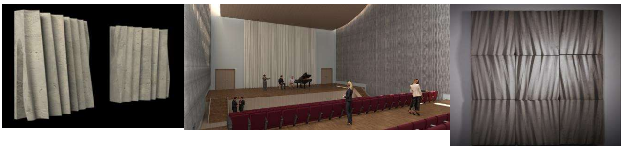
Figure 6 – Diffusive panel design Alpha. Left: object rendering. Middle: interior scene rendering. Right: finished product photo
