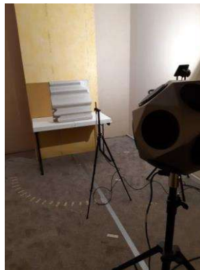
Figure 13 – Testing setup for diffusive panel ‘Beta’.
