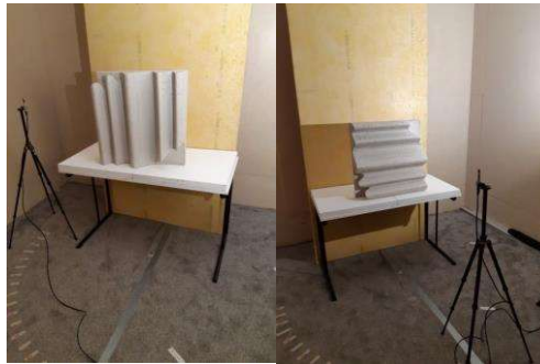
Figure 10 – Diffusive panels 'Beta'. Left: vertical shaped orientation. Right: horizontal shaped orientation.
