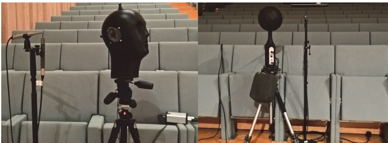
Figure 4 – Photographs of some of the measurement hardware. Left: omni and figure-of-eight mic set and binaural microphone. Right: omni mic and spheric acoustic camera.
