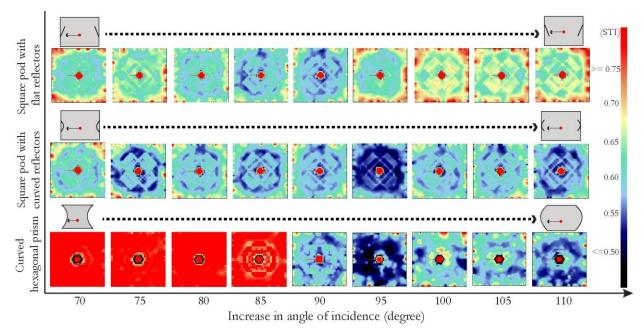
Figure 5 – Matrix B, Exploring the influence of angle of incidence on STI in three variations
