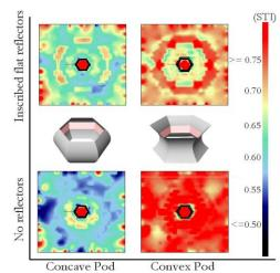
Figure 6 – The impact of flat reflectors on STI of concave and convex pod
