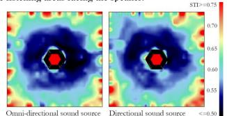
Figure 1– STI maps with directional vs. omnidirectional sound source
