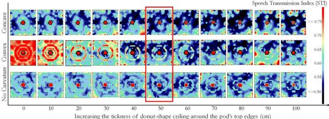
Figure 4 – Matrix A-2, Exploring STI maps of three types of the pods with wraparound donut-shape canopy of various sizes
