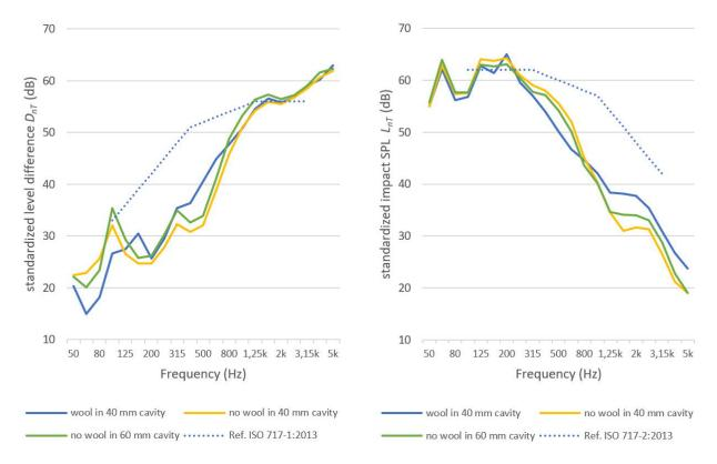
Figure 7. Measured airborne (left) and impact (right) sound insulation for the horizontal arrangement
