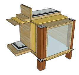
Figure 2. A 3D representation of the CLT prototype module (with adjacent elements)
