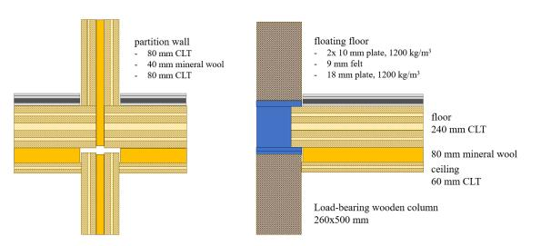
Figure 1. Wall, floor and ceiling constructions
