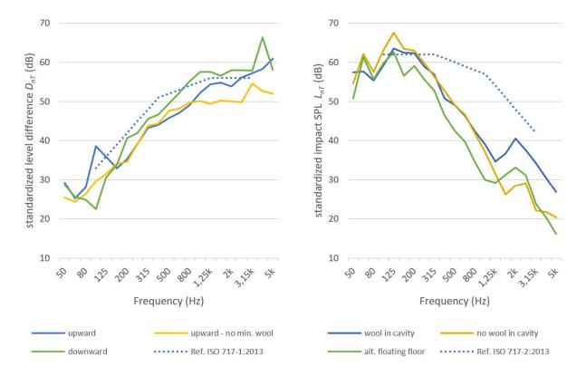
Figure 6. Measured airborne (left) and impact (right) sound insulation for the vertical arrangement
