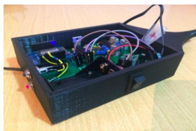
Figure 16 – Final design of the sound level meter.
