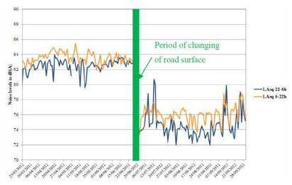
Figure 1 – Reduction of day and night noise levels near the source (median) after the pavement change.
