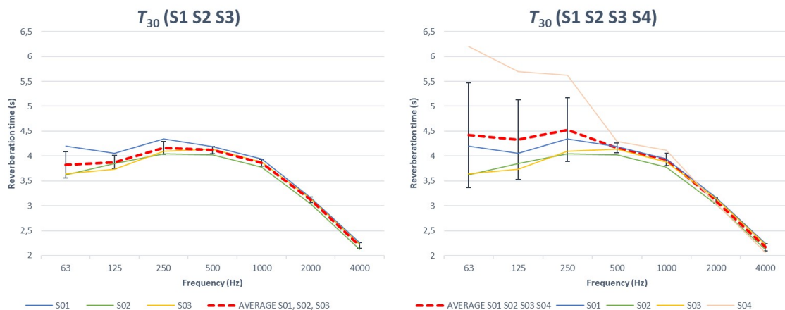
Figure 4– Graph showing reverberation times in the measured positions for sound sources S01, S02 and S03 (left) and for sound sources S01, S02, S03 and S04 (right) together with average values.
