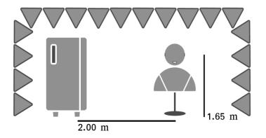
Figure 1 – Measurement setup used in recording reference signals and masking signals.
