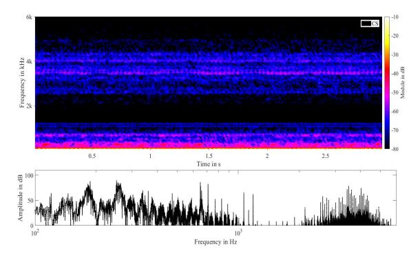
Figure 4 – Masking signal from the recording of a permanent refrigerator.
