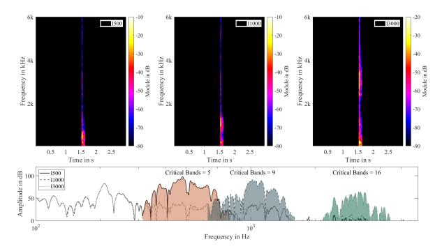
Figure 3 – Reference signals filtered with bandpass filters tuned to the central frequencies of 500 Hz, 1000 Hz and 3000 Hz.
