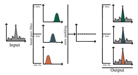
Figure 2 – Signal processing used for reference signals.
