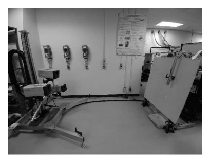
Figure 1 - Measurement setup for the determination of the dispersion relations in plywood. Panorama of the panel and the laser Doppler vibrometer, with detail of the clamping of the panel and detail of the fixing of the piezo.
