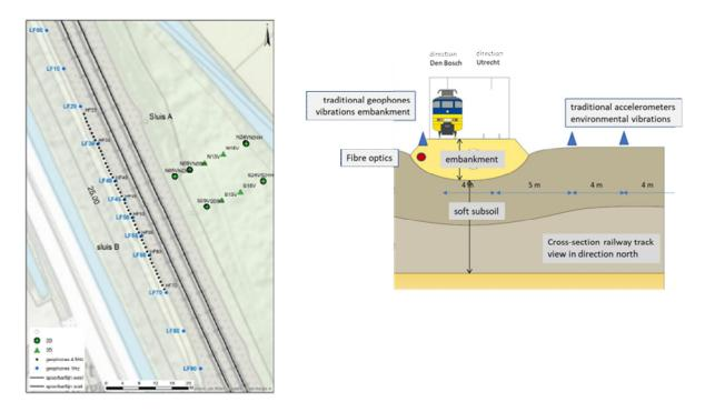
Figure 1 Overview of the measurement site south of Culemborg. Left top view, right cross-section looking in Northbound direction (from Den Bosch to Utrecht)
