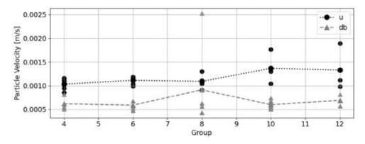
Figure 3 Vibration velocity Vmax of train pass-by's at 5 m (northbound <sup>…</sup>●<sup>…</sup> u) and 9m (southbound --▲-db) as a function of train length ((number of carriages per train) for train type VIRM double decker
