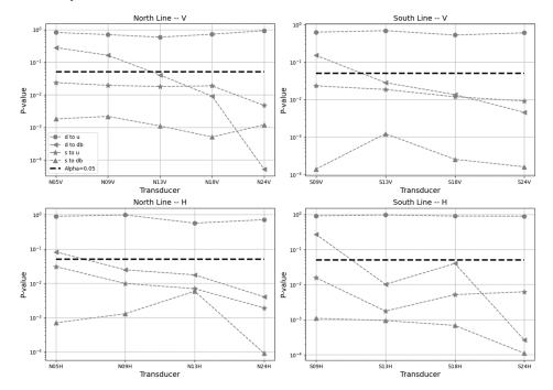
Figure 7 Critical values for hypothesis (H0 versus H1) on distance from the eastern track. Top the vertical vibrations, bottom the horizontal vibrations; left the north line, right the south line.
