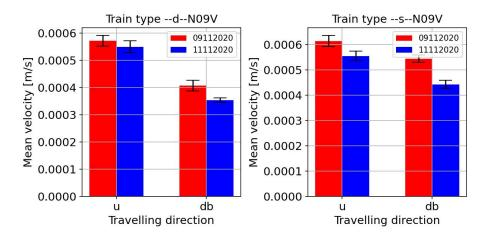
Figure 6 Comparison of maximum velocity for vertical vibrations over all train pass-by's before (red) and after (blue) maintenance works at signal N09V. See text for more information.
