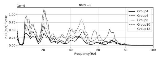
Figure 4 Power spectral density for vertical vibrations in point N05 for passing double decker, influence of train composition (group is number of wagons).
