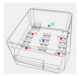
Figure 2– Virtual model of the classroom with the positions of the talker (St), the receiver (R), and the two (S1 and S3) and four (S1–S4) competing talkers.
