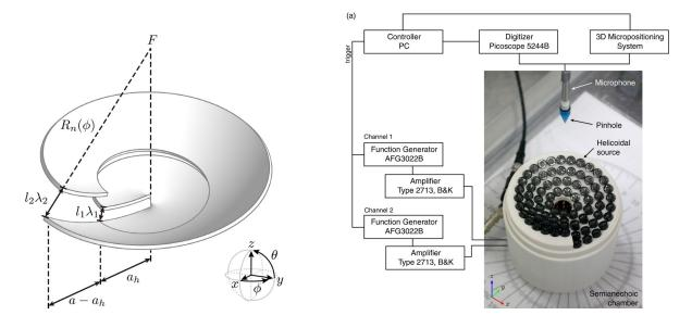
Figure 1 – (a) Scheme of the helical surface to focus two confocal vortex beams. (b) Experimental setup.
