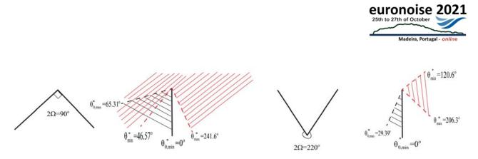
Figure 6: Ranges of source and receiver locations around the half plane  $\theta^*, \theta_0^*$  that correspond to all source and receiver combinations around a wedge of  $\Omega$ =45° and of  $\Omega$ =110°.
