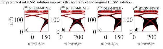
Figure 2: Contours of relative error with the exact BTMS solution of the mDLSM [(a)(b)] and of the DLSM solution [(c)(d)] at time  $\tau^* = 0.025(\bar{t}\gamma^2)$ . The terms  $p^{irf,i}$  and  $p^{irf,r}$  in the mDLSM and the DLSM are compared separately against the corresponding terms of the BTMS solution.
