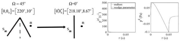
Figure 5: The impulse response and the N-wave response for the wedge configuration shown on the left is identical to the impulse response and the N-wave response constructed via Eq. (28) from the impulse response for the half plane configuration shown in the middle.
