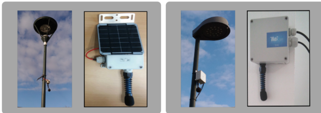
Fig. 2: The leaf (left) and gateway (right) sensors.
