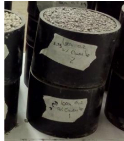
Figure 3 – Porous concrete samples, for impedance tube.
