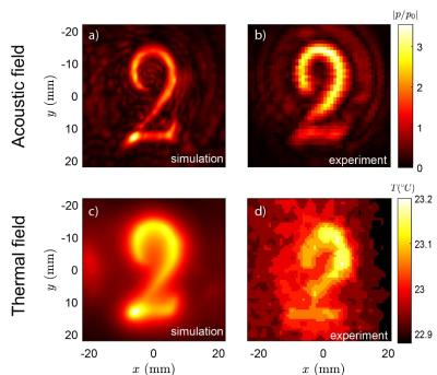
Figure 2. (a) Simulated acoustic pressure field. (b) Acoustic pressure field measured in degassed water. (c) Simulated thermal pattern in liver tissue. (d) Thermal pattern measured with an infrared camera in liver tissue.
