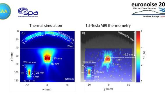
Figure 3: (a) Thermal simulation for a 1-cm wide hologram located at 65 mm from the transducer surface and (b) for the focused transducer without the lens. (c) MRI-thermometry measurement for the hologram and (d) for the focused transducer without the lens.
