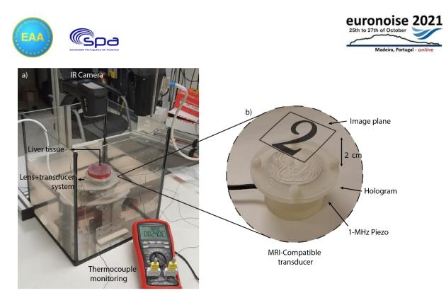
Figure 1: a) Experimental setup for thermal hologram validation using an infra-red thermal camera. b) Scheme of the employed lens-transducer system
