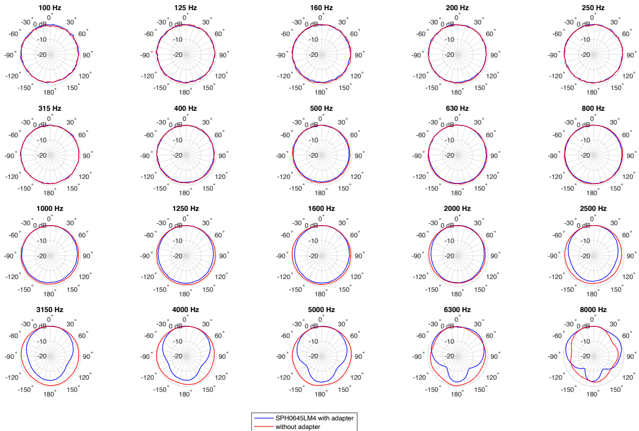
Figure 8: Directivity diagram in third octave band for SPH0645LM4H.
