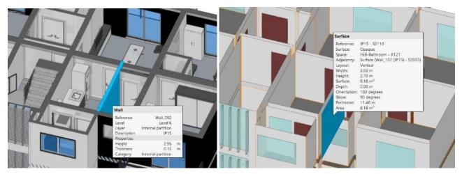
Figure 3 – Elements of the analytical model derived from the architectural model.
