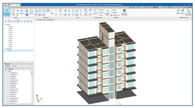
Figure 4 – Analytical model generation in Open BIM Analytical Model.
