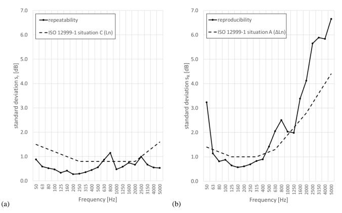
Figure 4 – Standard deviation under (a) repeatability and (b) reproducibility conditions for  $\Delta L$  of the vinyl floor covering.
