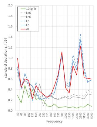
Figure 5 –Standard deviation under repeatability conditions for the different measurands determining  $\Delta L$
