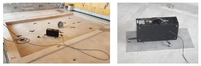
Figure 2 – Impact sound insulation measurement of bare floor and bare floor with vinyl floor covering
