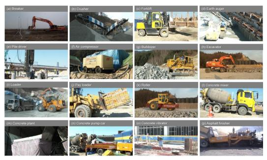
Figure 1 – Photos of sixteen construction machines.
