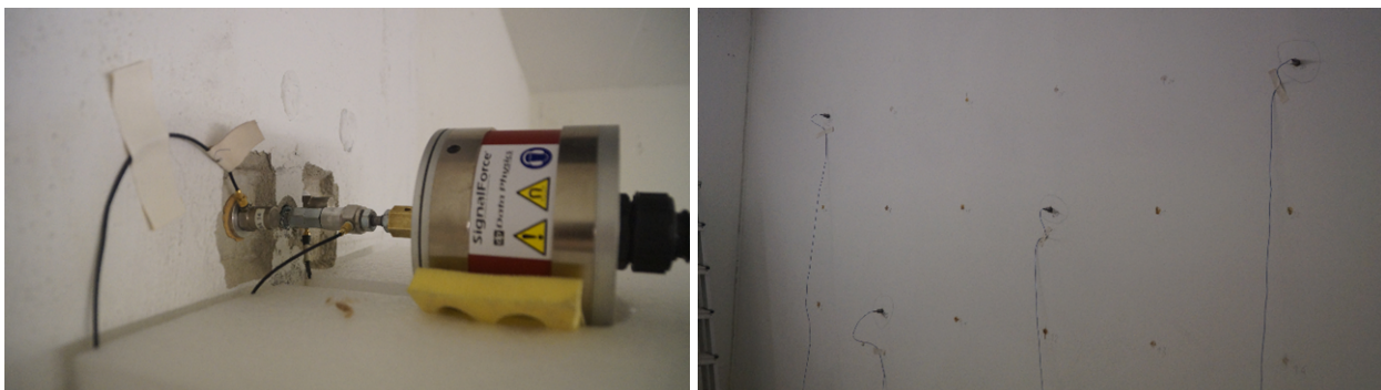
Figure 2 – Test set-up for the measurements with a reference structure borne sound source. Force and velocity (real part of the cross-power-spectrum) measured on the contact point of a shaker with the installation wall (left, source room). In addition, the average velocity of the wall (right picture) and the sound pressure level is measured in the receiving room.
