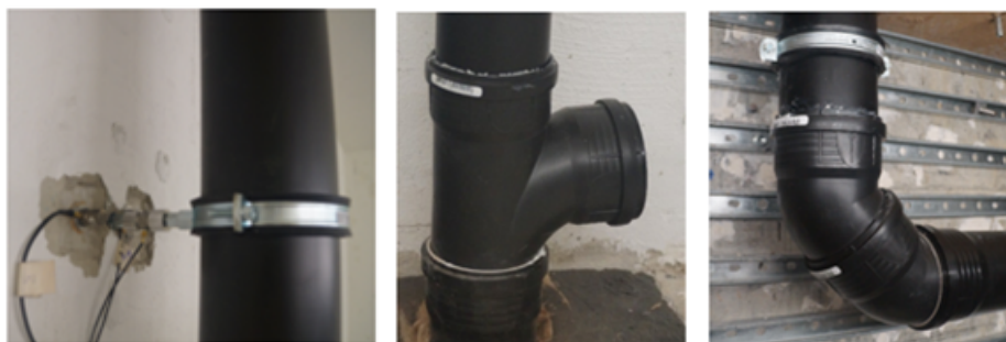
Figure 1 – Top left: Test facility with standard set-up for measurements according EN 14366 [1], [2]; (RR: receiving room, SR: source room).
