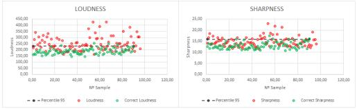
Figure 17. Comparison Correct/Defective Gearhead. Loudness and Sharpness.
