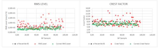
Figure 16. Comparison Correct/Defective Gearhead. RMS Level and Crest Factor.
