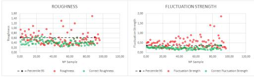
Figure 18. Comparison Correct/Defective Gearhead. Roughness and Fluctuation Strength.
