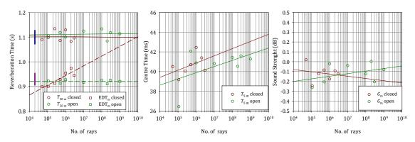
Figure 6. Behaviour of spectral averages, spatially averaged, of the acoustic parameters as a function of the number of rays for the open and closed model.
