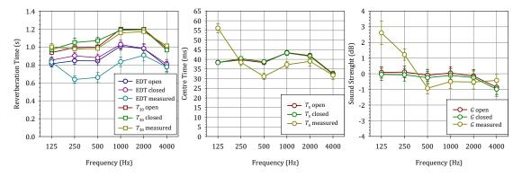
Figure 5. Comparison of the spectral behaviour, spatially averaged, of simulated parameters with the open and closed model and the experimental measures. Vertical bars value the spatial dispersion through the standard error.
