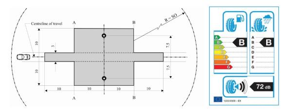
Figure 2. Left: a highly schematic representation of the noise coast-by test [9]. The shaded part represents the test area that is passed by the test vehicle. Two microphones are mounted, each (7.5  $\pm$  0.05) m away from the reference line (centre line of the test track) and (1.2  $\pm$  0.02) m above the ground. Source: Directive 2001|43|EC [2]. Right: example of a label for a C1 class tyre. Source: Reg. 122|2009 [8].
