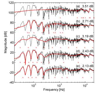
Fig. 7 - Parallel filter implementations of order 20 with different pole-positioning techniques. Graphs are scaled by 20 dB for clarity. The crosses indicate the poles frequencies.
