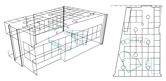
Figure 4 – Test room used for auralization. The number and position of acoustic elements were varied (type 1 – type 6).
