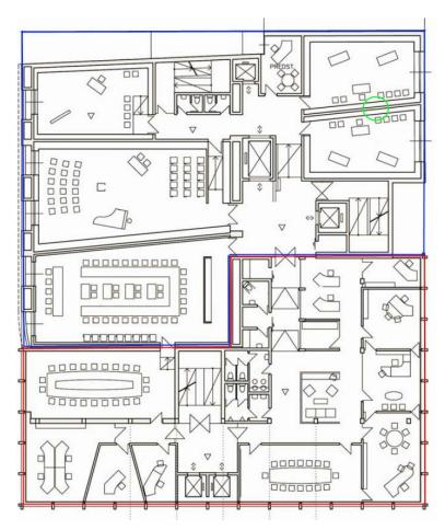
Figure 2 – Plan of the 3<sup>rd</sup> floor of the new building [12]. The old office building is shown in red, and the newly added part in blue. The green circle indicates a detail of a double wall construction.
