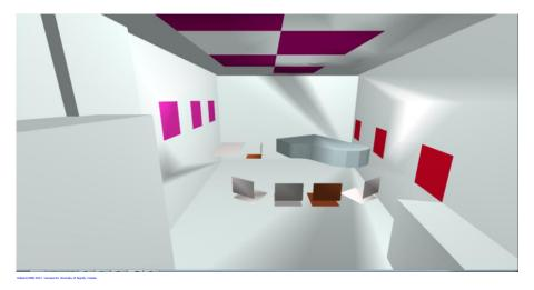
Figure 7 – Test room with additional 3 low freq. and 5 medium freq. absorbers on the walls.
