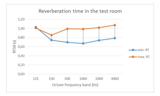
Figure 12 – Variations of the reverberation time in the test room with changeable acoustic elements. **4. CONCLUSION**
