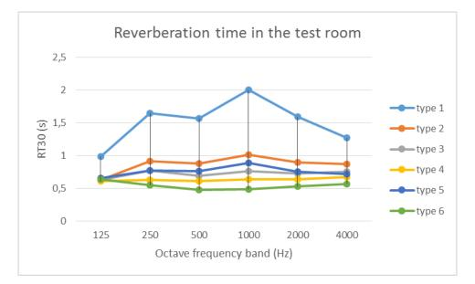
Figure 11 – Reverberation times of the test room depending on the type of acoustic finishing.
