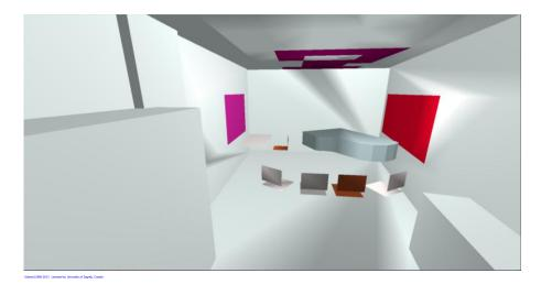
Figure 8 – Test room with 15 binary diffusers, 6 low freq. and 10 medium freq. absorbers.
