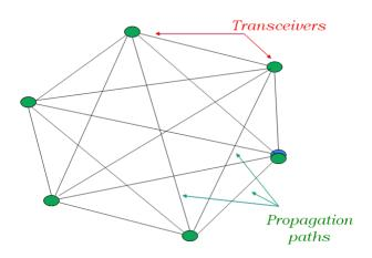
Figure 3.1. Schematic layout of an observatory related to ocean acoustic tomography
