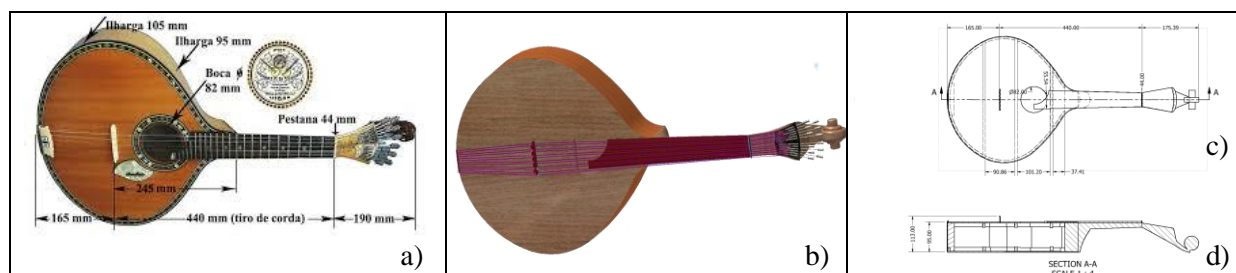
Figure 2 – a) Image of the Álvaro Merceano da Silveira’s guitar (source: [7]); b) image of the CAD model developed; c) front view of the model; and d) side view of the model.
