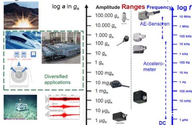
Figure 1 – Frequency ranges and amplitudes for accelerometer and AE-sensors.
