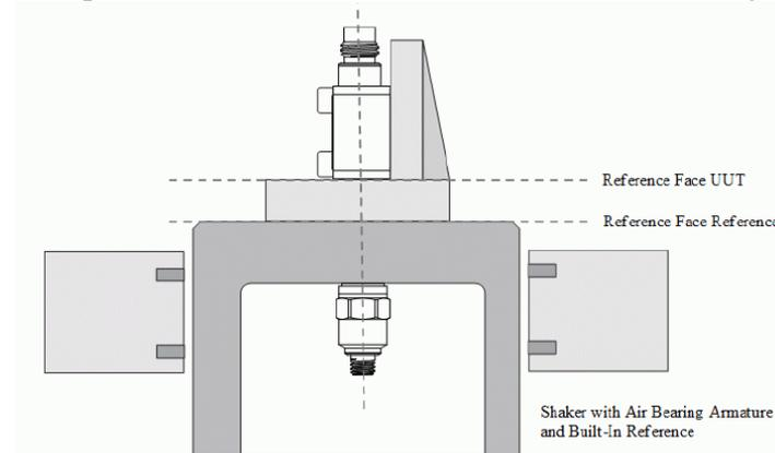
Figure 2 – View of a triaxial accelerometer as UUT. Mechanical adapter fixed to the calibration shaker air bearing armature. Built-in reference standard.
