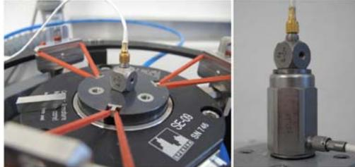
Figure 8a – Frequency response of a Kistler 8766A500AB triaxial accelerometer along x and z axes directly mounted to reference (results in Fig. 9).
