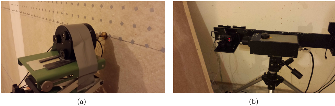
Figure 7: Measurement equipment. (a) Shaker that was used to excite the wall; (b) scanning laser Doppler vibrometer (developed in-house).
