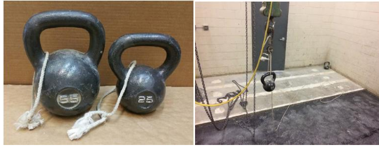
Fig. 8 – (a) typical dumbbells weigh and, (b) drop weight test set up used in RAL
