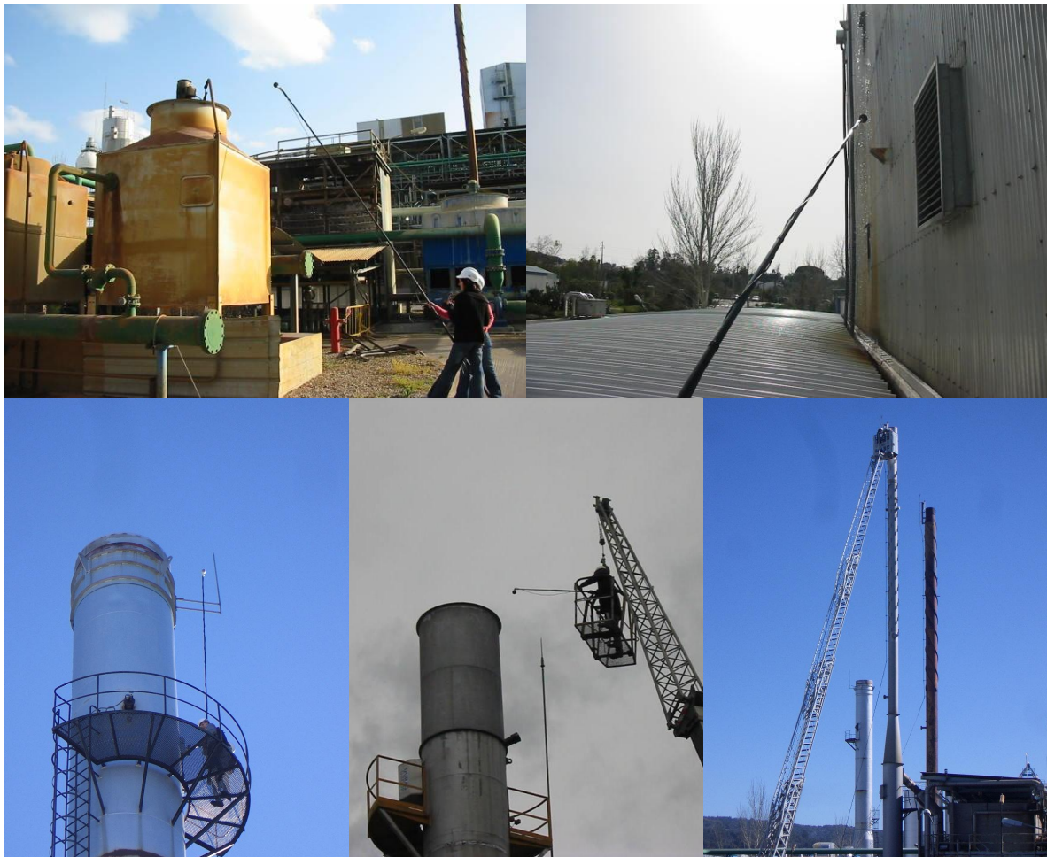
Figure 2 – Getting input data for the acoustic model of a factory: close field measurements.
