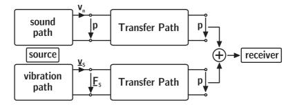
Figure 1 – Simplified block diagram of transfer path synthesis (after [1])
