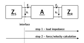
Figure 6 – Two-port as a central coupling element of TPA (after [1]).
