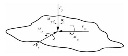
Figure 3 – Point contact of a source with complex description of the force transmission, three orthogonal forces and three moments (after [2]).
