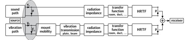
Figure 5 – Detailed block diagram of binaural transfer path synthesis (after [1])
