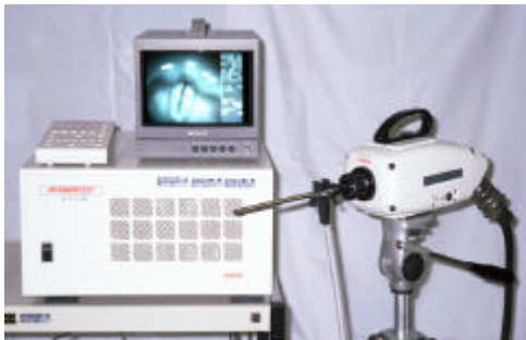
Figure 1. A picture of the camera head with an obliquely angled solid endoscope and a digital image memory with a video monitor. (Kiritani, 2000)
