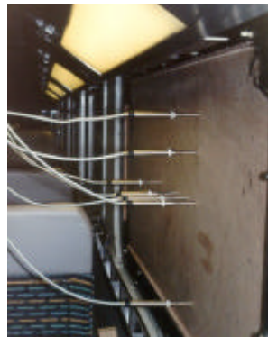
- Figure 3 : 7 wall pressure microphones arranged crosswise on the face of the TGV -
