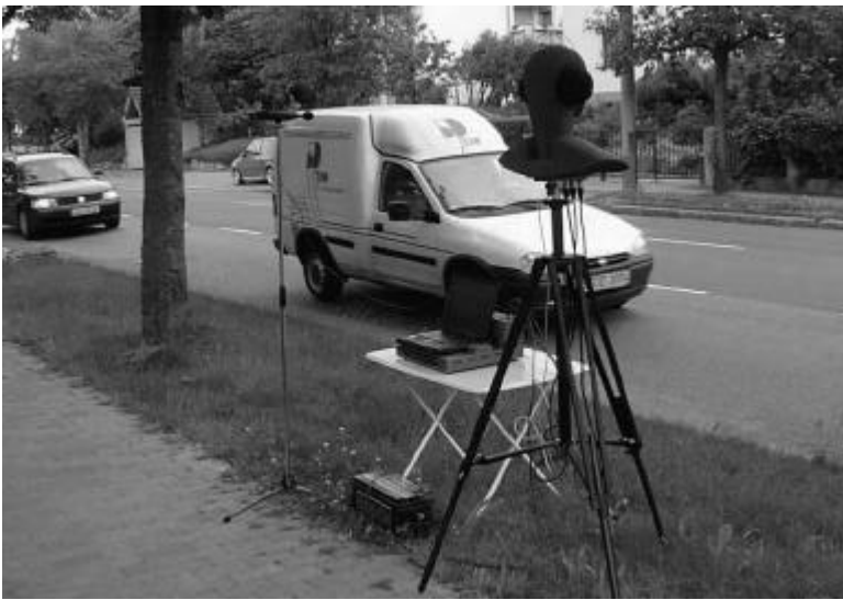
Picture 1: Set-up for Measurement at 2 Metres Distance in built-up Area
