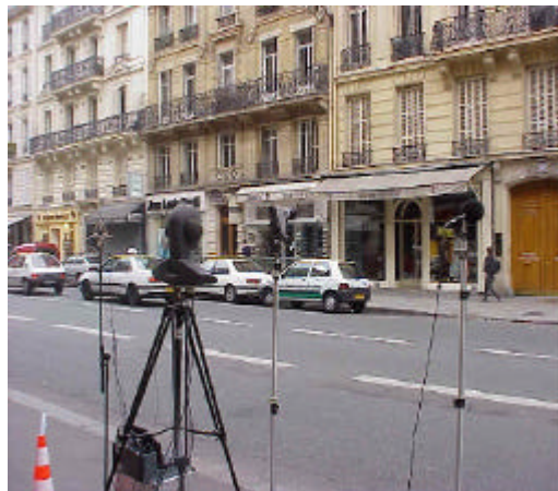
Fig. 2.- Typical arrangement for traffic noise recording
