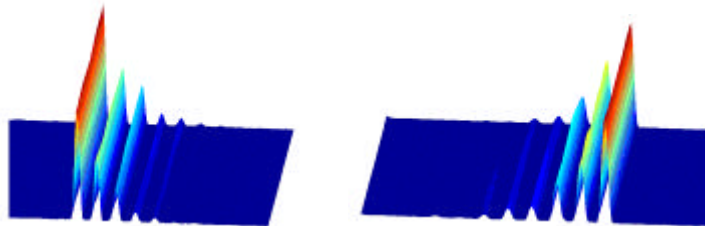
Figure 3 Highly resolved zoom-FFT spectra (100 spectra) of a slowly-moving reflector (about 0.002 \text{ ms}^{-1} ). Left: ( 19\text{kHz} - 2.5 \text{ Hz} \dots 19 \text{ kHz} + 8.7 \text{ Hz} ) moving away from the source, right: ( 19\text{kHz} - 8.7\text{Hz} \dots 19\text{kHz} + 2.5\text{Hz} ) towards the source. The spectral resolution is 25 \text{ mHz} . The largest intensity originates from the 19 \text{ kHz} carrier frequency.
