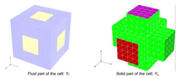
For that porous medium we consider that solid is isotropic. The porosity is 0.648 and the physical values considered in this academic test for the fluid and the solid are
