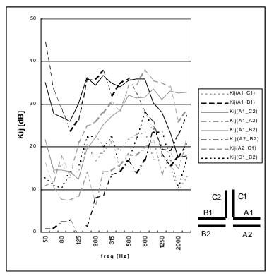
Figure 5 Vibration reduction indices as measured in experimental set-up 1
