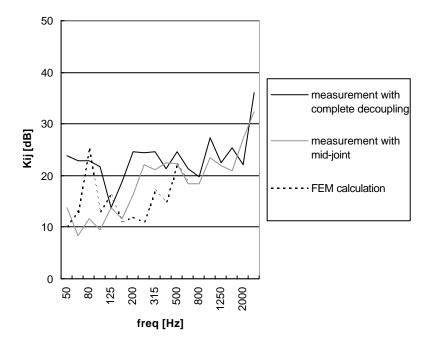
Figure 6 Vibration reduction indices as measured in experimental set-up 2
