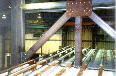
construction element were expected. This set-up was based on the FEM model more or less. In this set-up vibration reduction indices concerning the path floor – steel supporting structure – floor have been measured for two variants of the set-up.
