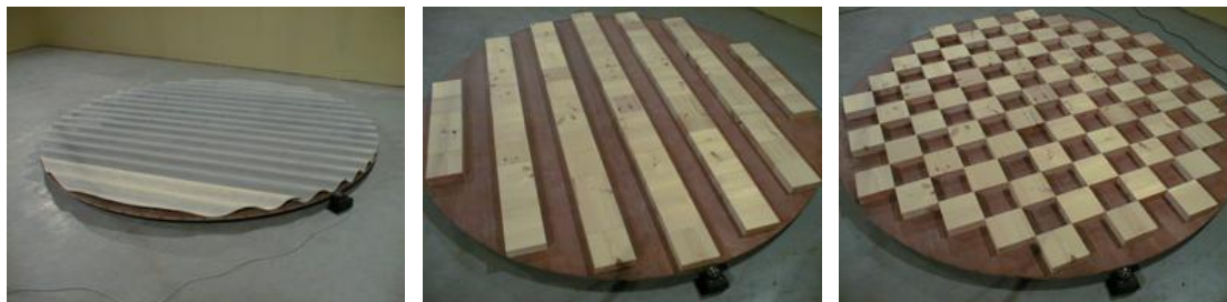
Figure 2: (a) Sine profile, (b) 1D-diffuser and (c) 2D-diffuser mounted in the reverberation room. The black box at the bottom right is the motor.
