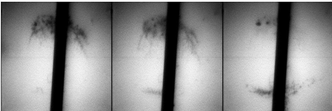
Fig. 2: Three pictures from a high-speed movie (2250 frames/sec; background 1 microsecond flash illumination; picture width approx. 1 cm each). The double layer has been "attached" to a hypodermic needle to better fix it in space for recording. The beat between flash light frequency and acoustic driving frequency highlights the antiphase oscillation of top and bottom part of the structure.
