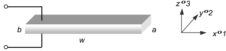
Fig. 2. Geometry of the piezoceramic element vibrating in a transverse (width) mode.
